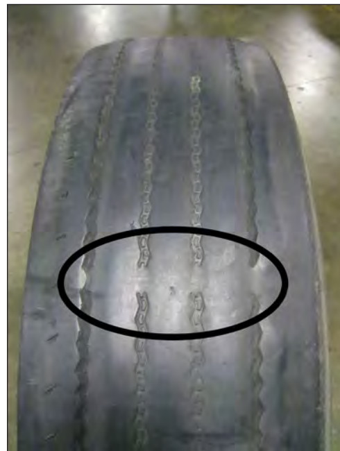
FIGURE 19: Tread Wear Indicators
