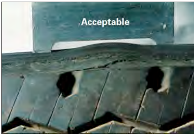
FIGURE 51: Section Repair Bulge (Less than 3/8")
