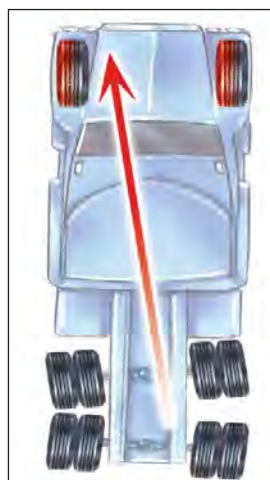
FIGURE 35: Left Thrust - The drive axles push the truck left. Shoulder wear occurs on the left side (outboard) side of the left front tire. Shoulder wear also occurs on the left (inboard) side of the right front tire.
