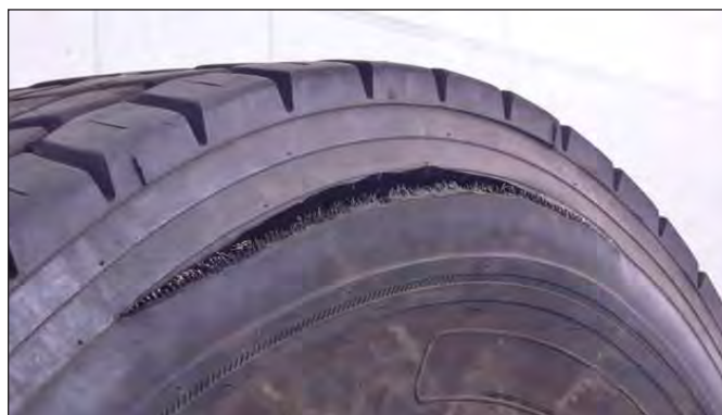
FIGURE 21: Example of a Zipper Rupture
