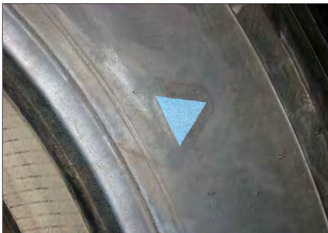
FIGURE 53: Blue Triangle Patch Applied to Sidewall
