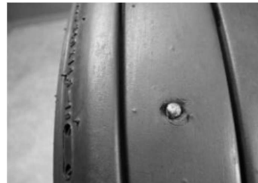
FIGURE 2: FOD Tire Damage Example
