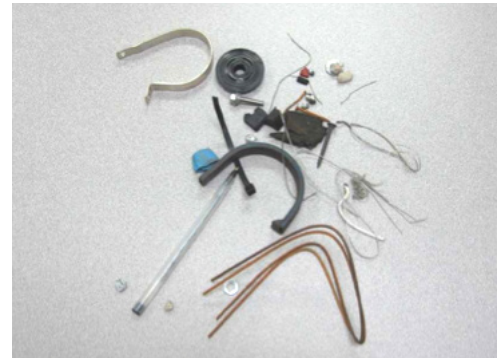
FIGURE 1: Typical Operating Area FOD
