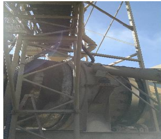
INJECTED THROUGH RAP COLLAR
