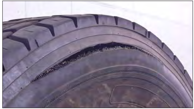
FIGURE 21: Example of a Zipper Rupture
