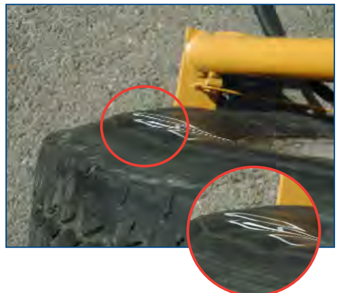
FIGURE 28: Undulating Rippled Sidewall 21
