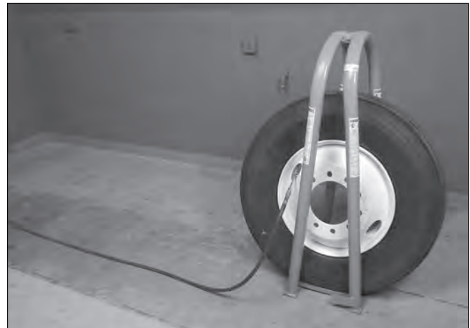
FIGURE 25: This is just one type of restraining device available for tire service facilities. With the valve core removed, inflate tire using a clip-on air chuck with a pressure regulator and an extension air hose.
