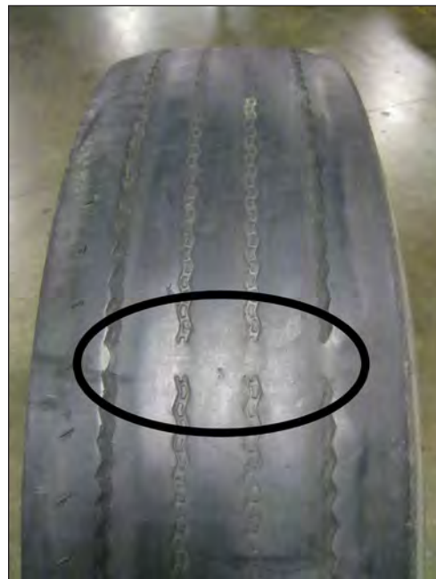
FIGURE 19: Tread Wear Indicators
