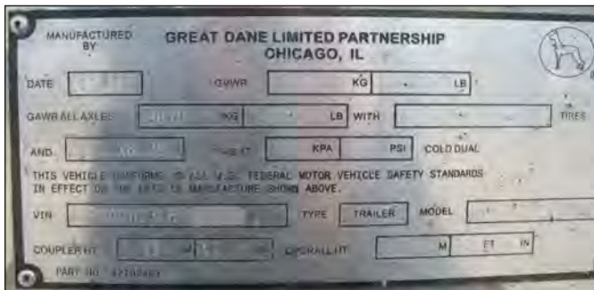
FIGURE 10: Trailer Certification Label
