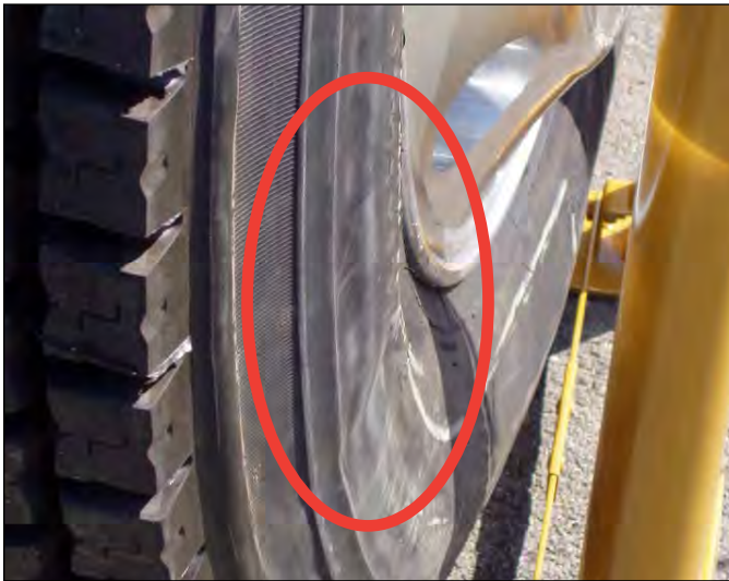
FIGURE 26: At 20 psi, you can begin to see the presence of distortions in the sidewall of this truck tire (circled in red). Due to a heavier sidewall construction, bus and refuse tires would present this condition at 40 psi.
