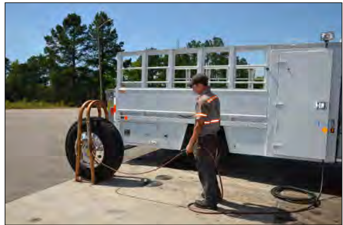
FIGURE 17: Inflating in Portable Safety Cage
