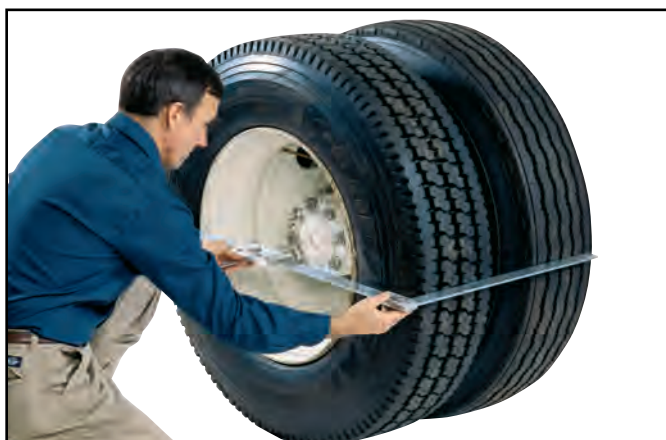
FIGURE 47: Dual Tire Meter
