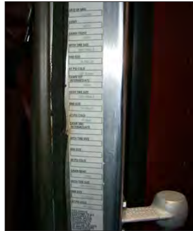
FIGURE 11: Truck Certification Label
