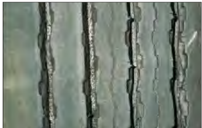
FIGURE 60: Regrooved Tire Tread Edges
