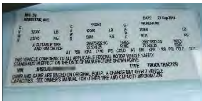
FIGURE 44: Truck Certification Label
