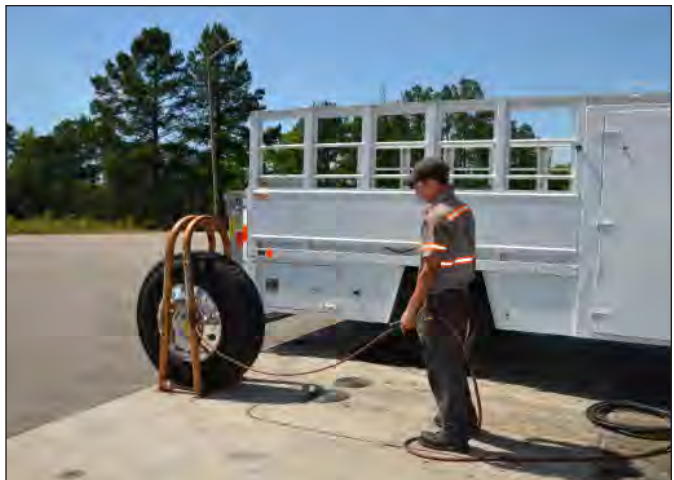
FIGURE 64: Inflating in Portable Safety Cage
