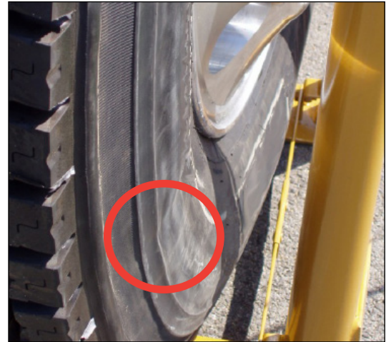
FIGURE 7: At 20 psi, you can begin to see the presence of distortions in the sidewall of this truck tire (circled in red). Due to a heavier sidewall construction, bus and refuse tires would present this condition at 40 psi.
