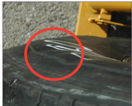
FIGURE 9: Visible sidewall condition indicative of a pending “zipper rupture.” Note the undulating rippled sidewall.
