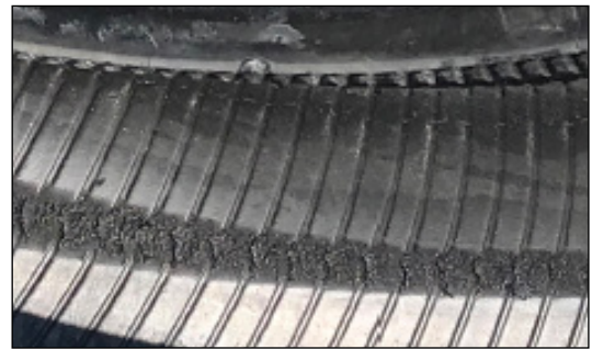
FIGURE 3: Note the abraded area on the tire innerliner. This condition is the result of the tire being operated under inflated and/or overloaded.
