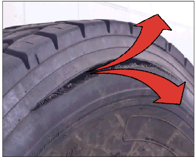
FIGURE 1: Zipper Rupture Example
