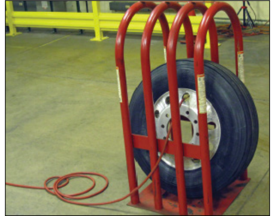
FIGURE 5: This is just one type of restraining device available for tire service facilities. With the valve core removed, inflate tire using a clip-on air chuck with a pressure regulator and an extension air hose.
