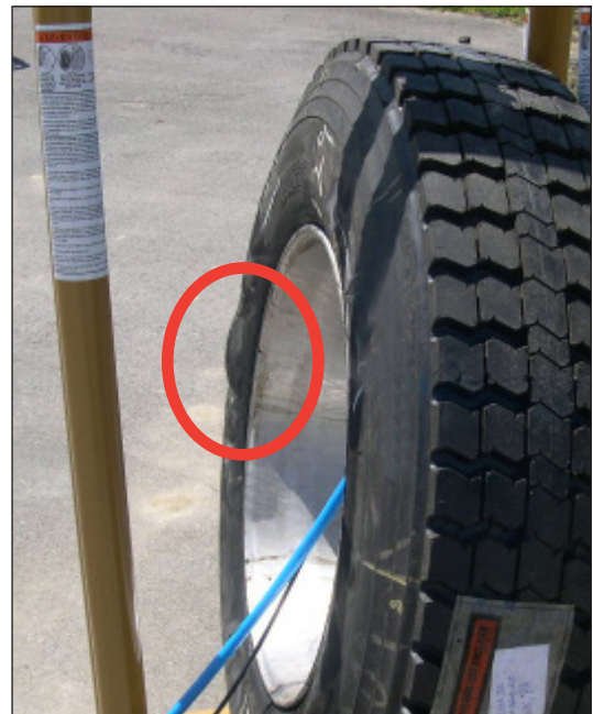
FIGURE 8: Visible sidewall condition indicative of a pending “zipper rupture.” Note the bulge in the sidewall.
